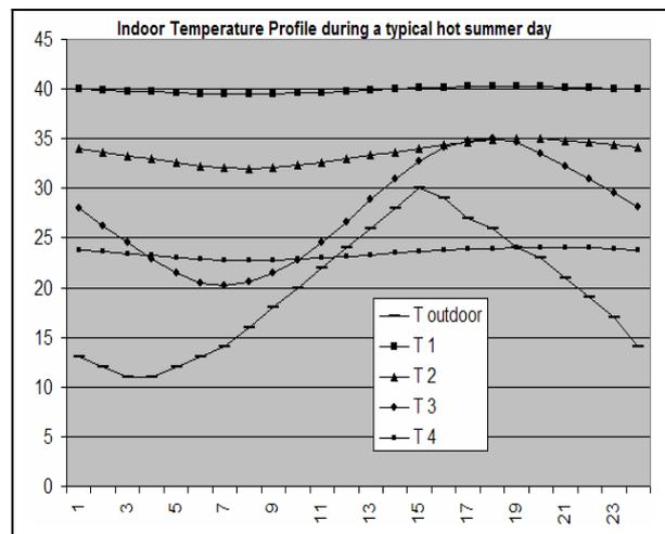
**Figure 9:** Indoor temperature profile during a typical hot summer day: T1 – Heavy construction without night cooling, envelope closed during the day, north orientation and overhang, T2 - Heavy construction, night cooling, west facing and overhang, T3 – Light construction, north facing without overhang. T4 – as constructed with heavy construction, night cooling, north facing, natural ventilation during the day
