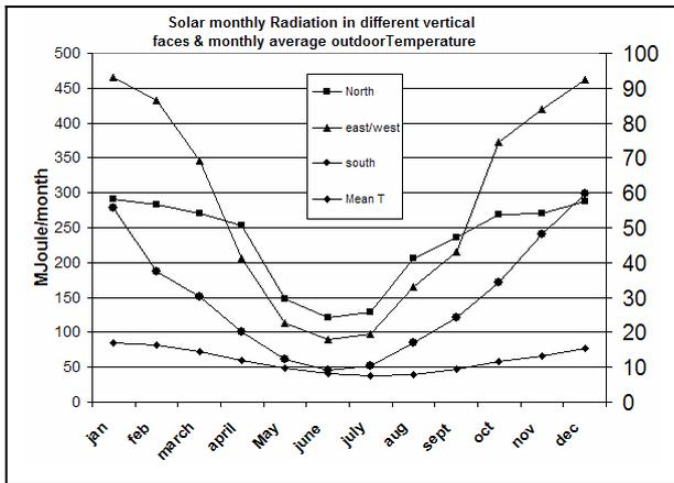
Figure 4: Solar monthly radiation in different vertical faces and monthly average outdoor temperature
